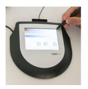
The configuration of the brightness of the device is carried out via the service menu. Tap on the desired setting ('darker' or 'brighter') by using the pen supplied.
