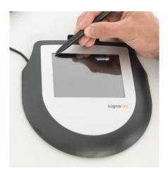
Touch the display with the pen at the **top left-hand corner**. While holding the pen reconnect the pad to the power supply. After booting successfully, the LED switches from red to orange.
