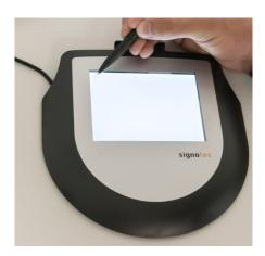
As soon as two intersecting narrow lines on a white background appear at the top left- hand corner of the display, tap the center of the intersecting lines by using the pen.
